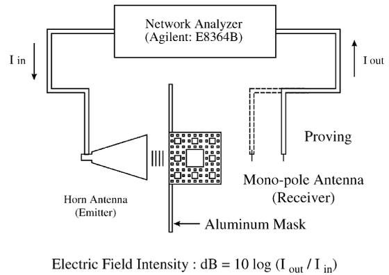
Fig. 2. An experimental configuration to prove the intensity profile of the electric field inside and outside the Menger-sponge structure.
