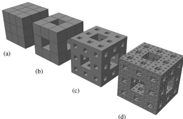
Fig. 1. Schematic illustrations of three-dimensional fractals with a Menger-sponge structure: (a) stage 0; (b) stage 1; (c) stage 2; (d) stage 3.
